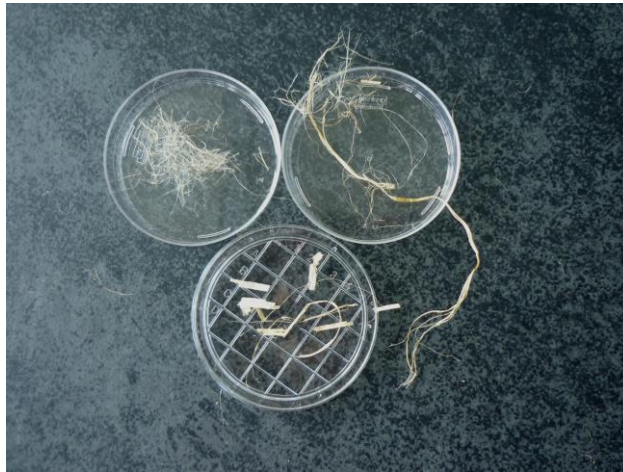
Figure 6: Fractions of the hemp samples after manual separation
