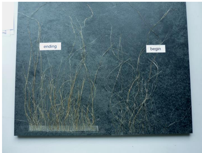
Figure 5: begin and ending of aligning the fibre bundles at the end
