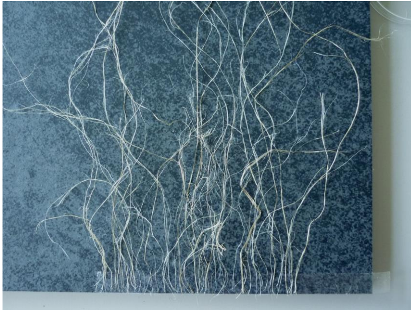
Figure 2: Hemp fibre bundles aligned at one end (fibre bundle collective)
