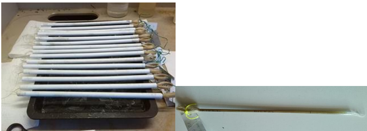
Figure 2: Composite samples (35 cm long) from the pultrusion process; left: hackled hemp in the PTFE mould; right: hemp fibre-reinforced composite rod.
