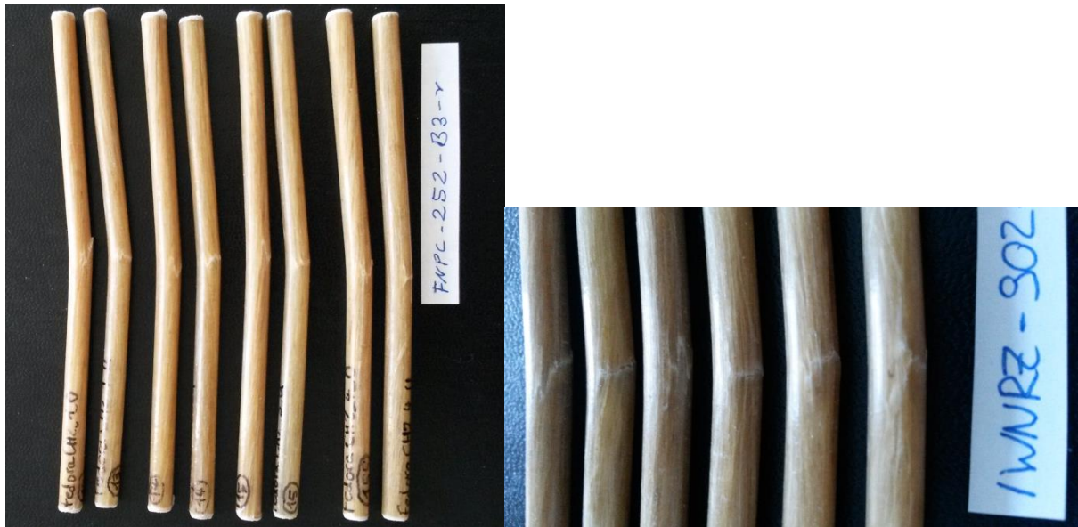
Figure 5: Characteristic damage at the tensile side of the test specimens after bending.
