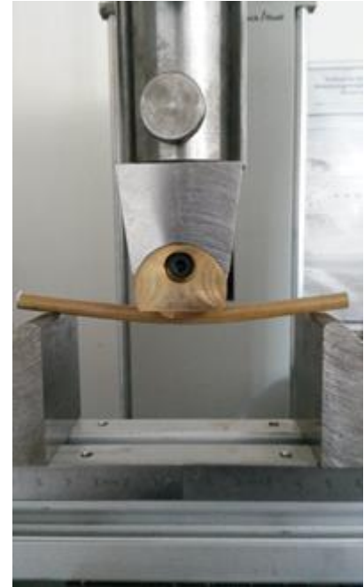
Figure 3: Setup for bending tests
