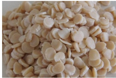
Figure 3. Hemp-reinforced PLA granules from hackling losses; samples show no thermal degradation and the yellowish colour of the hemp fibre bundles after bio-degumming is still present in the granules.
