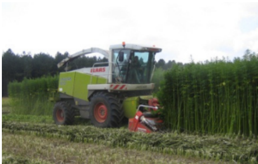
Figure 8: Harvesting system HempCut 3000/4500
